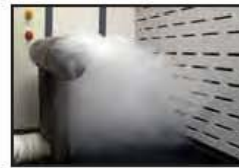
Smoke released inside the hood moves in a horizontal stream to the primary baffle slots.
